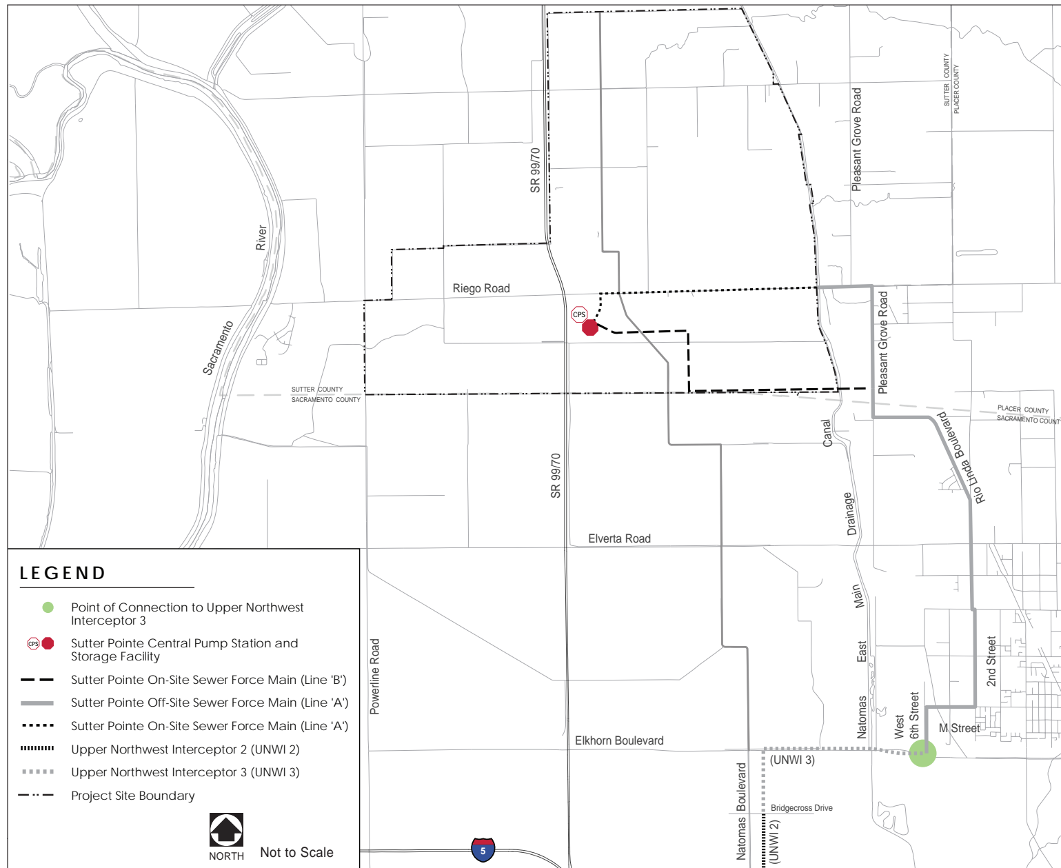
Exhibit 9.4: Backbone Sewer Plan (Off-site)
